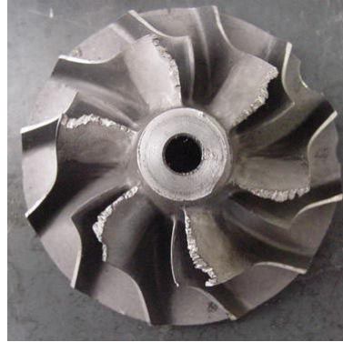
FIGURE 2.2: Damaged impeller, performance turbochargers (2013)
