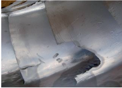
Fig.1 Erosion damage of Francis runner in Peru
