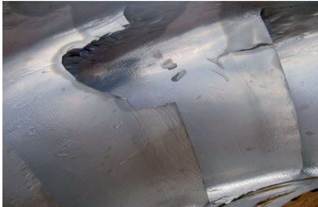
Figure 3: Erosion on outlet region on the runner vane, Cahua Power Plant [4]
