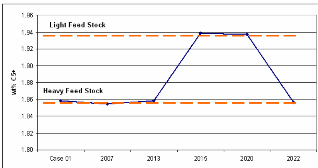
Figure 29: Light and heavy feedstock set points for LPG in De-Propaniser
