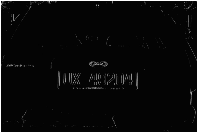
(c) Edge image using system framework calculation of HSV, and using v from HSV as pixel value.
