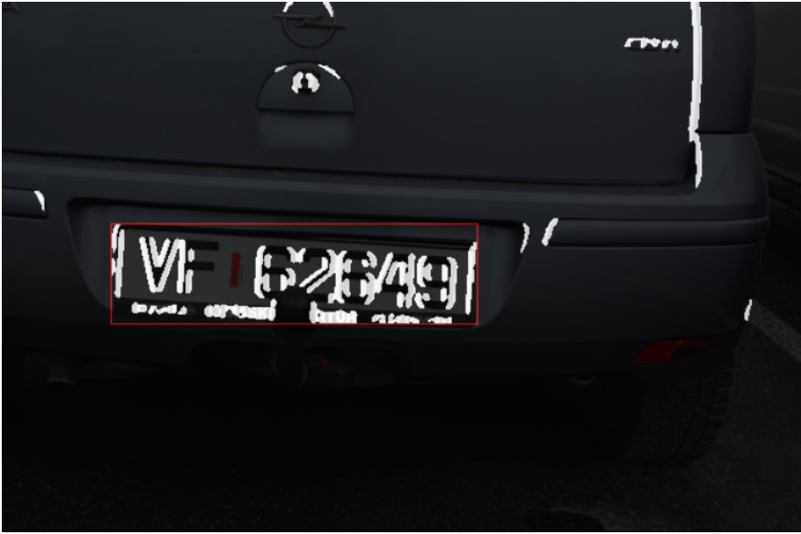
Figure 5.1: License plate location using color difference edge image.
