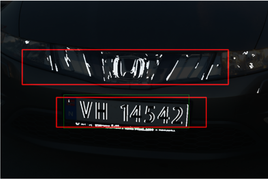
Figure 6.3: Example of false positive detection by Color difference edge image filtering.
