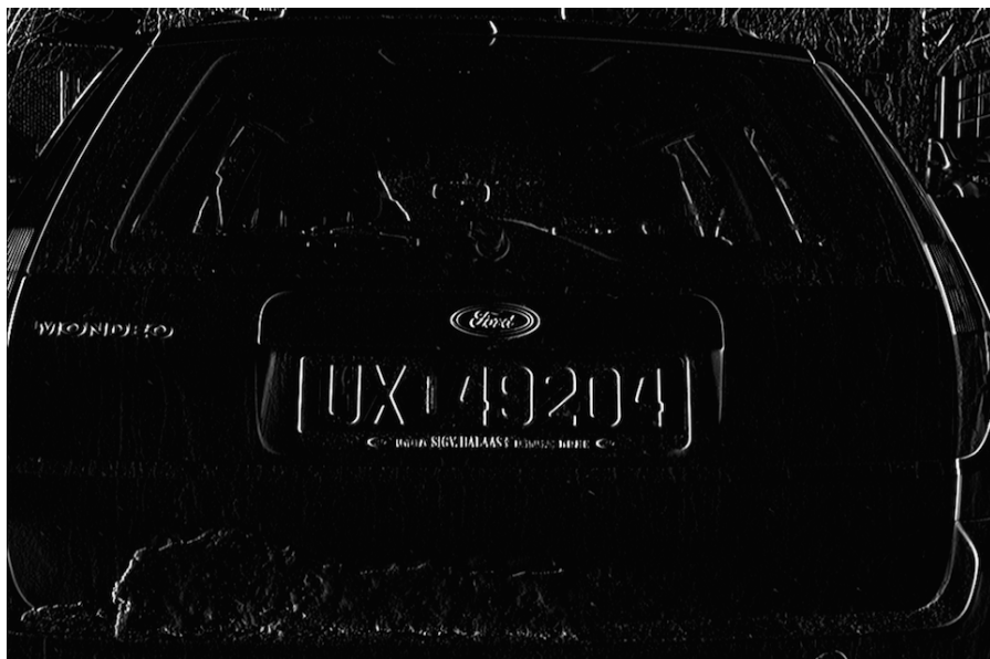
(b) Image after convolving with vertical Sobel kernel.
