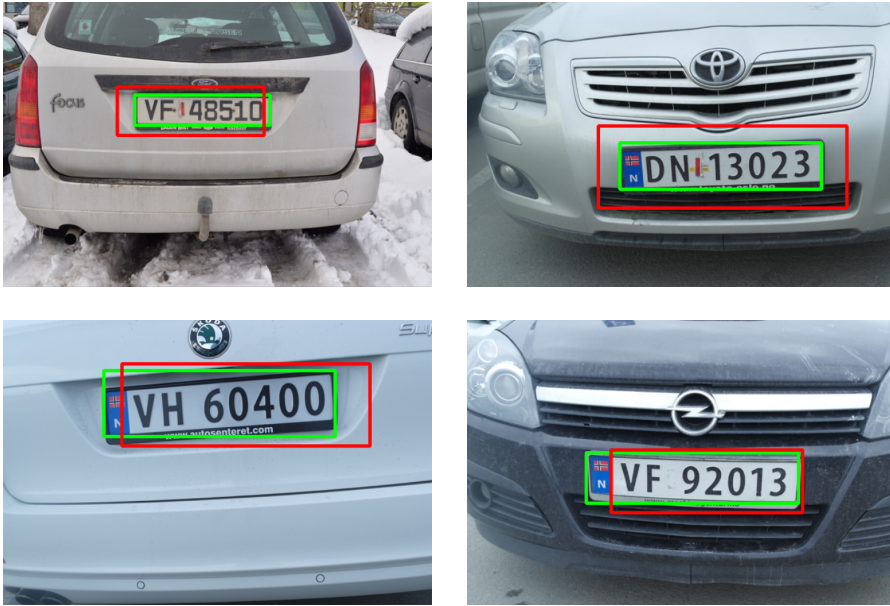
Figure 6.2: Examples of cascade classifier detections. The green rectangles represent the correct rectangle for the LP, the red rectangles represents the detected rectangle.
