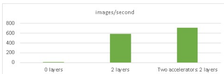
Figure 5.3: Performance when processing only layer 1 and 2, and subtracting DMA initializations.
