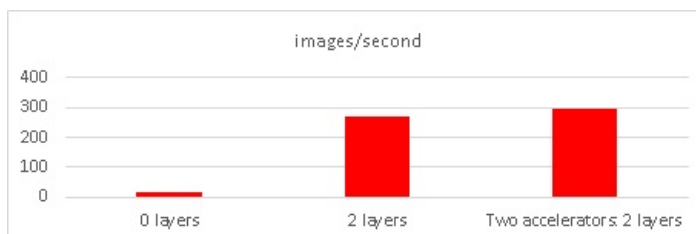
Figure 5.2: Performance when removing layer 3 and 4 from the network. I.e. only processing layer 1 and 2.
