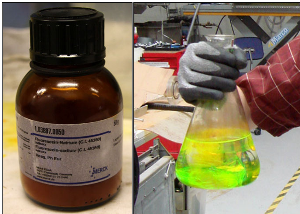
Figure 5.2 – Fluorescein-Natrium can (left) and colored water (right).
