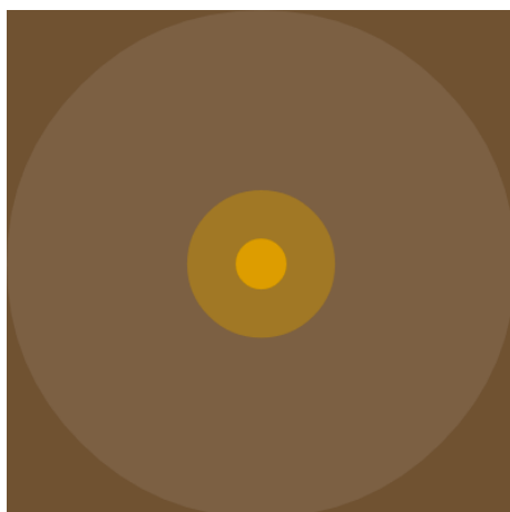
FIGURE 3.9: A detail view of the circle, illustrating the three parts: the outer touch area indicator, the resizable level indicator, and the inner position indicator.
