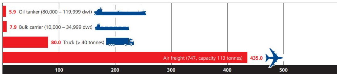
Figure 1: Emission in grams CO 2 per tonne-km from different modes of transport (International Chamber of Shipping, 2014; Buhaug et al., 2009).
