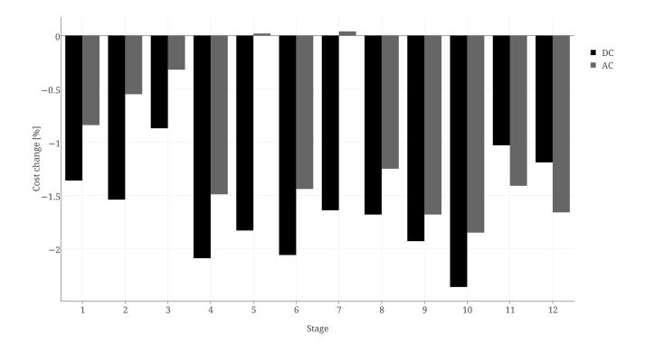
Figure 5.3: DC switching actions applied to ACOPF - GB network
