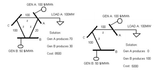
The OTS is a reformulation of the DCOPF or ACOPF problem, where a binary variable  $\lambda_k$  is introduced.  $\lambda_k$  returns 0 when line k is fully in service and 1 when line k is removed from the system. The solution provides the location of switches under a given operational scenario. When introducing the binary variable  $\lambda_k$  to the ACOPF problem presented in (2.3)-(2.9), we get the following formulation of the AC-OTS problem:
