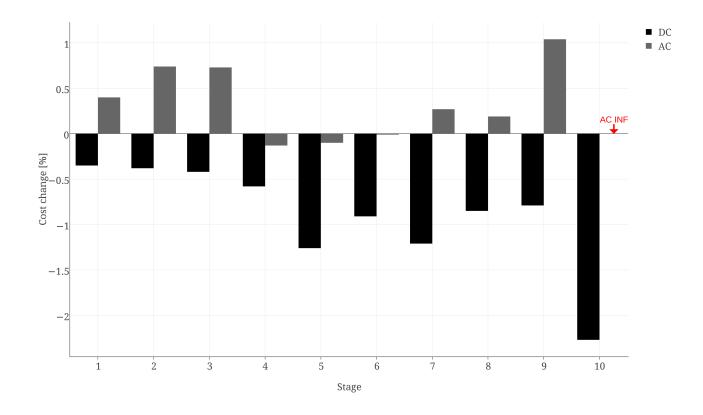
Figure 5.1: DC switching actions applied to ACOPF – case118
