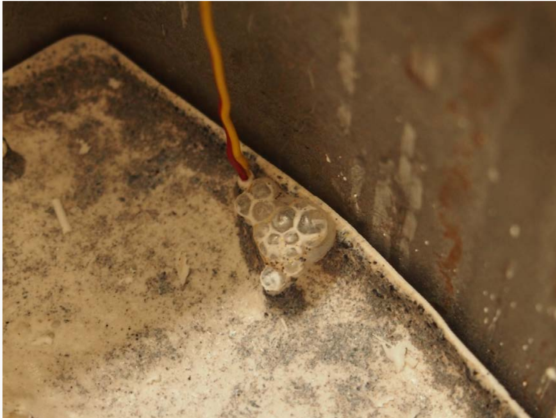
Figure 15 – Bubbles possibly due to impurities in the melt
