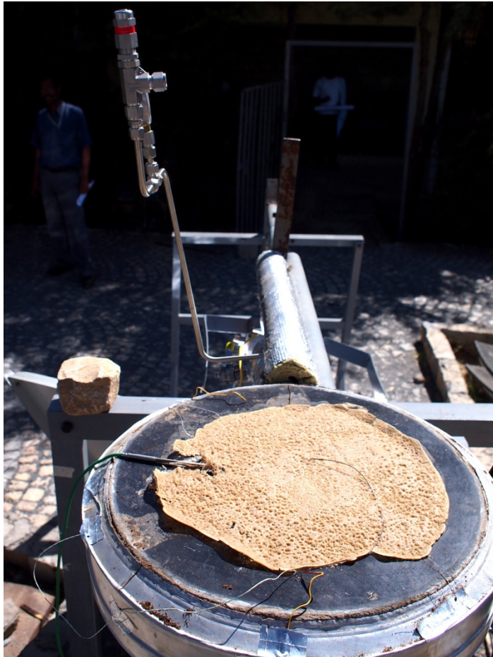
Figure 12 - Injera baked on solar powered steam heated stove
