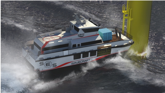
Figure 9: Example of a SES design: Umoe Mandal WaveCraft [83].
