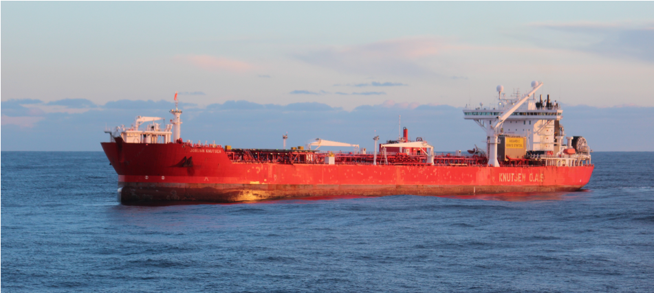
Figure 2.2: A storage ship for condensate, Åsgard C, seen from an OSV. Photo: Nils B. Albjerk, February 2015.
