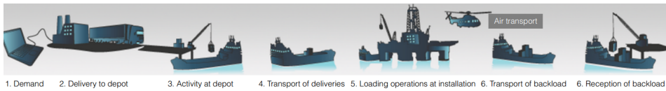
Figure 2.3: The process of supplying offshore installations. Illustration: Statoil (2015c).
