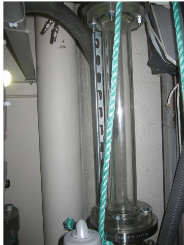
Figure 8: Acrylic pipe for flow visualization
