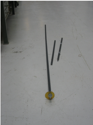
Figure 7: Pig for draining the test section
