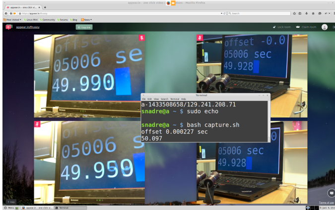
Figure 4.1: An example screenshot from a Firefox test run on node A. The nodes are, from top left and clockwise, A, C, B and D. We can see how the \approx 33 ms refresh rate manifests itself, as the visible times are .928, .959, .990, and 0.021 (node A, barely visible behind the .990).
