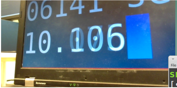
Figure 4.2: A screenshot where a node has sent two overlaying timestamps. In this case interpreted as 10.106, which is reasonable as it's close to the expected \approx 33 ms increase from the previous 10.075.
