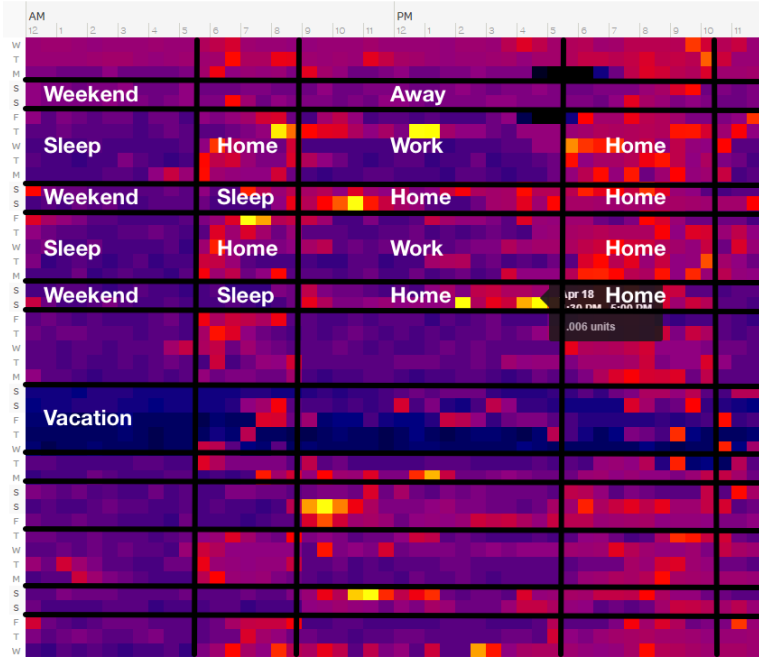
Figure 4.2: Heat map of power usage versus time. The power company can deduce a lot about its users by using simple analysis. Original heatmap without analysis by: Powershop Australia Pty Ltd
