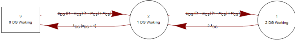
Figure 9.6: Markov dependability model of the smart grid including a power grid control system and stress propagation between DGs.
