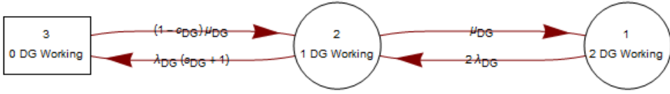
Figure 6.4: Markov dependability model of the smart grid system from Figure 4.1 including stress propagation between DGs and repair crew telecommunication dependency.
