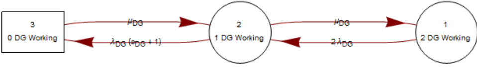
Figure 6.3: Markov dependability model of the smart grid system from Figure 4.1 including stress propagation between DGs.
