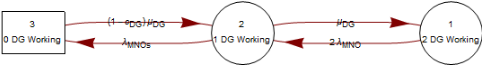
Figure 6.9: Markov dependability model of the smart grid system from Figure 4.1 including stress propagation between DGs, repair crew telecommunication dependency, and BS power backup.
