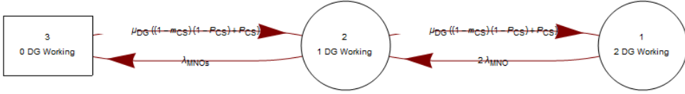
Figure 9.11: Markov dependability model of the smart grid system from Figure 4.1 including stress propagation between DGs, BS power backup, a power grid control system and repair crew telecommunication dependency.
