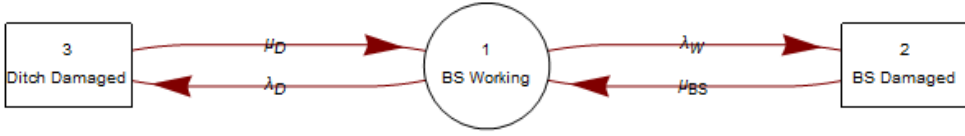
Figure 11.1: Markov dependability model of a single BS system with BS failures caused by normal weathering and a cable ditch for the BS.
