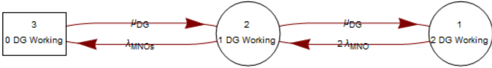
Figure 6.8: Markov dependability model of the smart grid system from Figure 4.1 including stress propagation between DGs and BS power backup.
