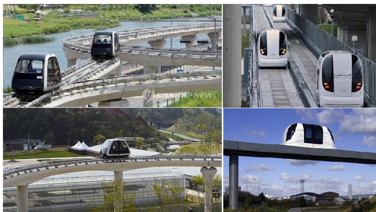
Figure 2.2: Picture of the Vectus(left) and ULTra(right) PRT systems. The pictures are taken from Podaris ??, PRT Consulting ??, connect2edmonton forum ?? and Upriser ??
