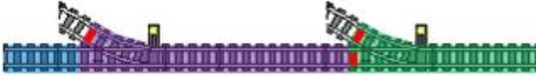
Figure 11.2: The division of sections at merging intersections. The sections are divided the same way as number series, but in contrast to number series, there must be one new section per merging intersection. While the blue and purple sections are in the same number series, the green is in another divided by an adjustment sleeper.
