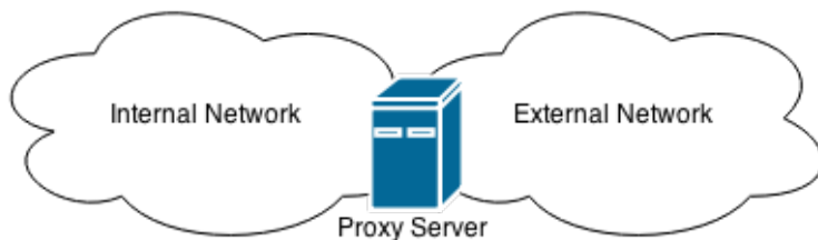
Figure 7.1: Network layout of the simulated ISP experiment, where the Proxy Server acts as a gateway between the two networks
