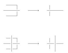
The first of these is exactly an  $R^2$  move, and the third is exactly an  $R^3$  move. The second is what is sometimes known as an  $R^0$  move, namely a manipulation of a diagram which does not affect the crossing information.
