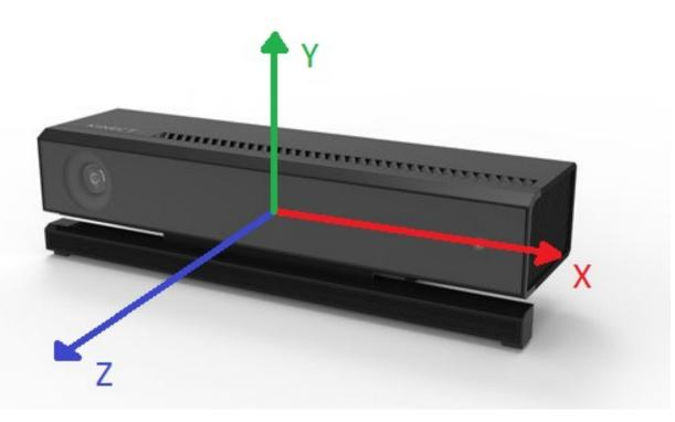
Figure 4.12: Kinect coordinate system
