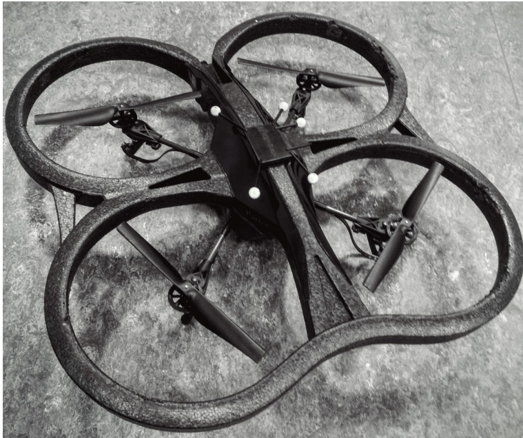
Figure 3.3: Photograph of the AR Drone 2.0 with reflective OptiTrack markers attached
