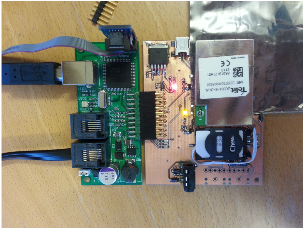
Figure 3.8: The new 3G board milled out, together with a universal board.
