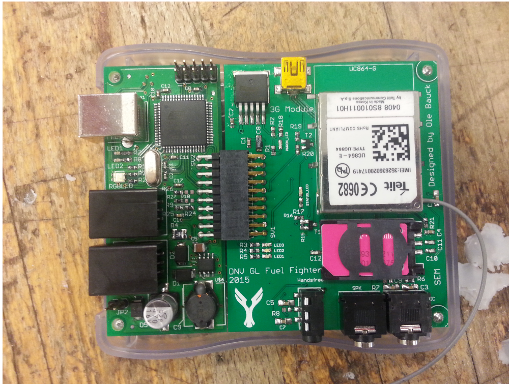
Figure 3.9: The final 3G module used in the car.
