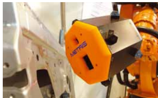
High scanning accuracy is guaranteed, as K-Robot eliminates the influence of robot warm-up, drift and backlash.
