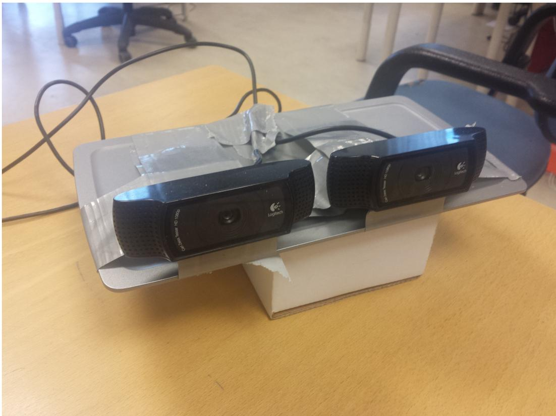
FIGURE 3.10: Stereo rig
