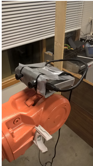
Figure 16: Due to low compatibility between the cameras and the tool plate on the robot it was attached with duct tape.
