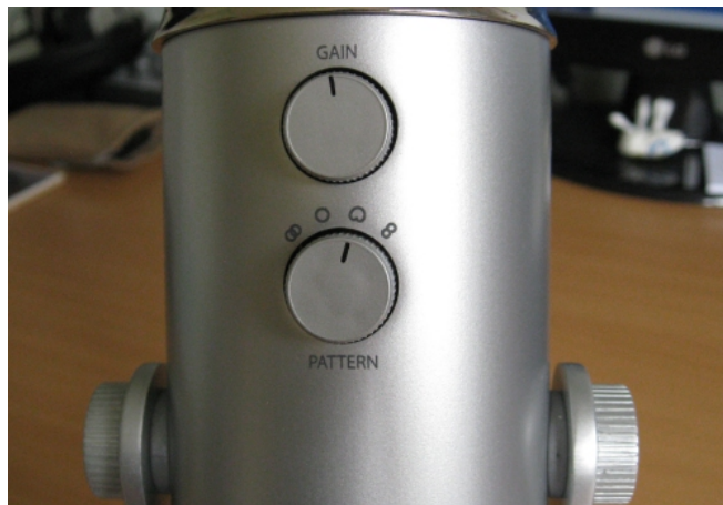
Figure 18: The backside of the microphone shows the gain and the four modes which are available: stereo, cardioid, omnidirectional and bidirectional.
