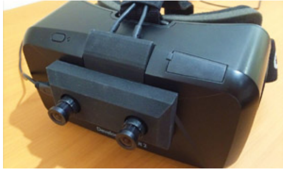
Figure 13: The intended use of Ovrvision is to bring the real world into the rift screen.
