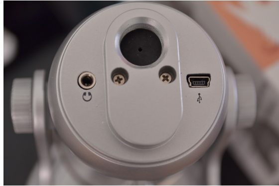
Figure 17: A mini-jack and USB connection is available from the bottom of the microphone.
