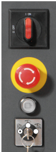
Figure 10: The control panel on the controller.
