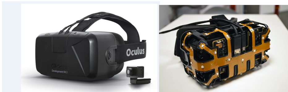
Figure 3: A picture of the Oculus Rift with and without the case. In the picture without the case you can see the led lamps that provides positional tracking. The camera reads the pattern of the leds, and based on this information it calculates the position of the headset.
