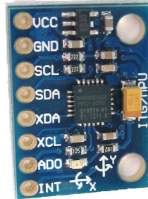
Figure 2.5: IMU used in our quadcopter
