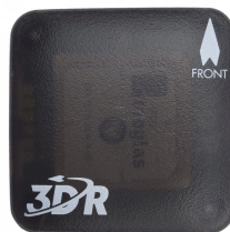
Figure 2.8: GPS used in our quadcopter
