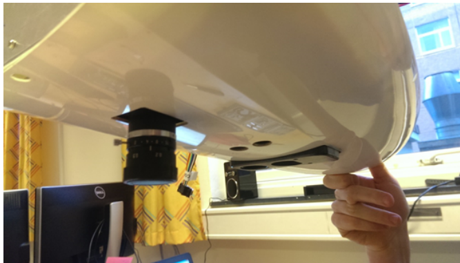
Figure 4.1: Camera placement in the UAV. It points straight towards the ground as long as the UAV has zero roll and pitch.
