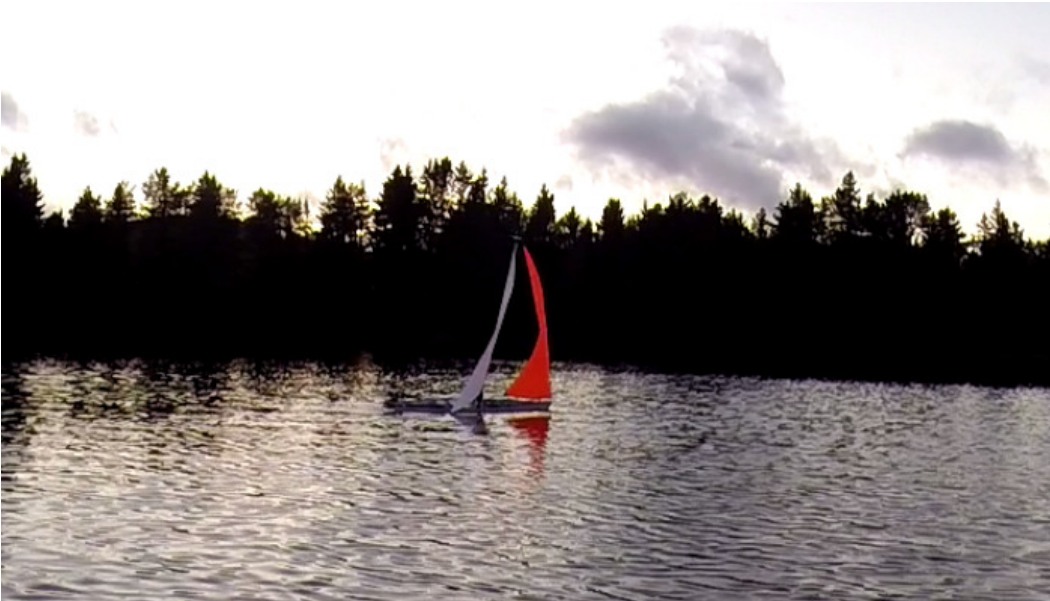
Figure 7.12: The boat in "heading hold mode". The main sail angle is clearly released outwards by the controller in order to make the boat turn right away from the wind.
