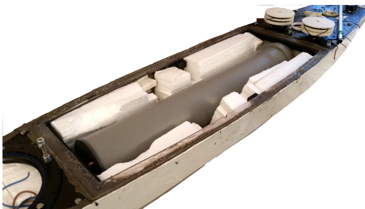
Figure 3.7: The housing placement within the hull.
