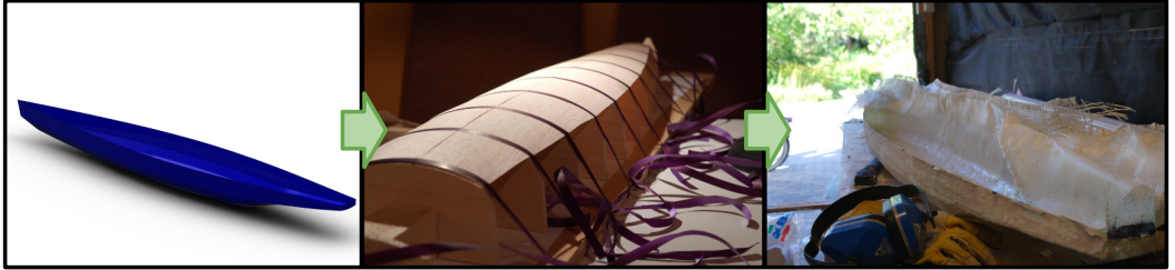
Figure 3.3: The hull casting process.
