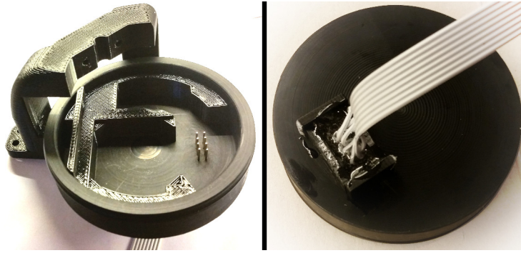
Figure 4.6: Wire seal and brackets for the housing assembly.
