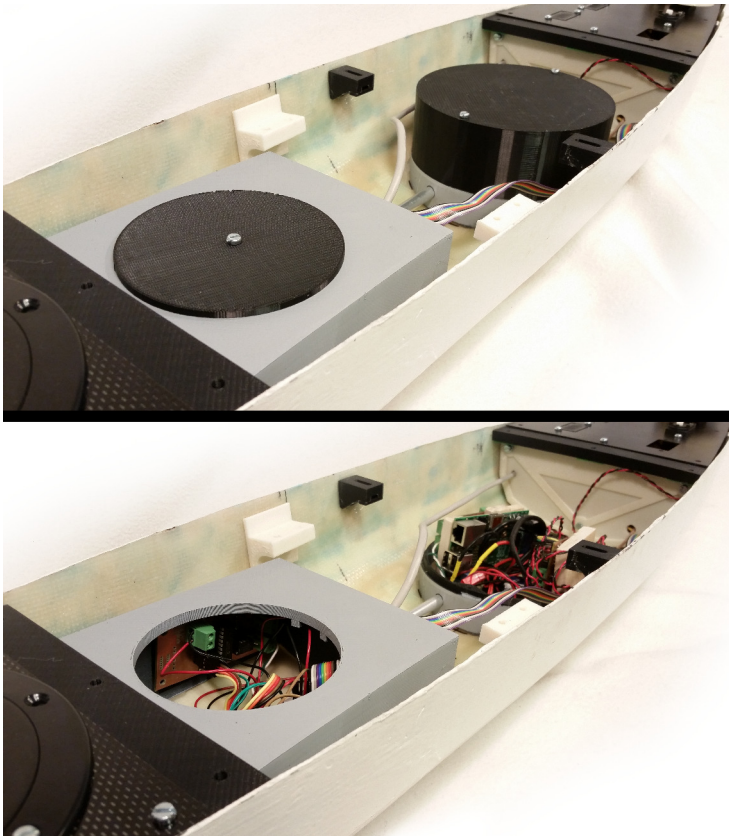
Figure 3.5: Redundant waterproof compartments.
