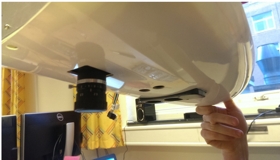
Figure E.2: Payload module is placed such that camera is pointing downwards
