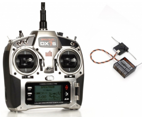
Figure 3.4: The Spektrum DX7s with its receiver. Image by courtesy of hobbyfly.com.
