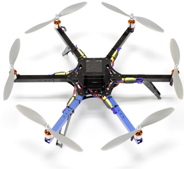
Figure 3.2: The ArduCopter 3DR Hexa B. Image by courtesy of 3drobotics.com.
