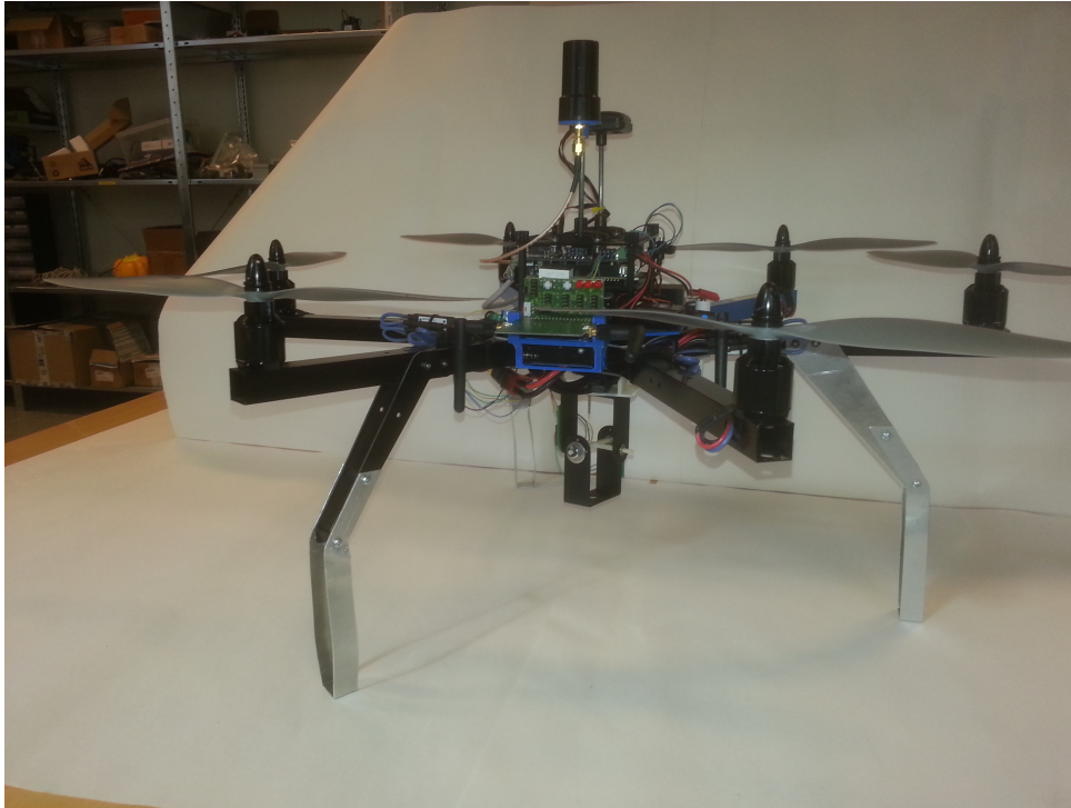
Figure 5.18: The hexacopter is used during the suspended load experiments. The suspended load is attached at the sensors below the multirotor system. The legs are elevated to protect the sensors during take-off and landing.
