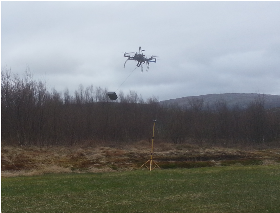
Figure 5.21: The hexacopter in the air with suspended load. Strong wind casts could push the system and load away. However, the multirotor controller was able to stabilize the system.
