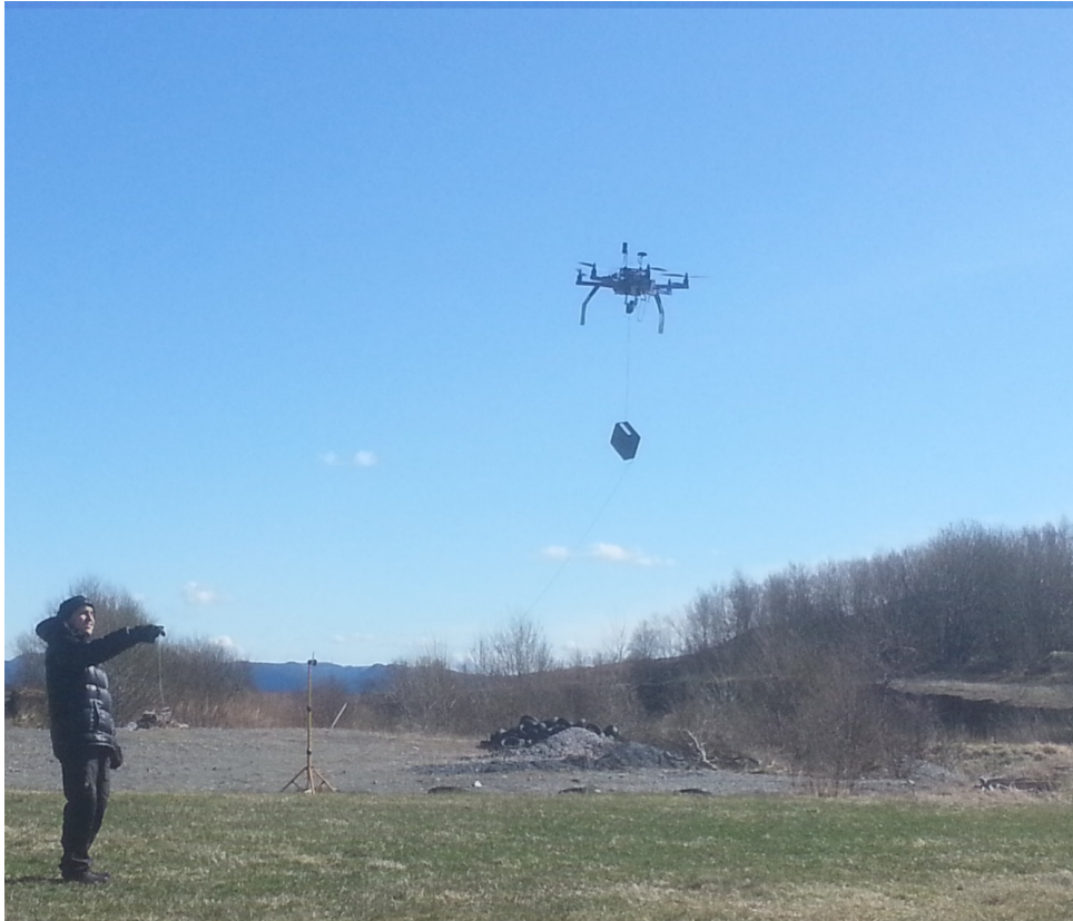
Figure 5.3: A picture from initial experiments with suspended load. The operator induces swings by pulling a rope that is attached to the load. The load weights 0.4 kg and attached 0.7m below the multirotor. The multirotor is on loiter mode during the experiments.
