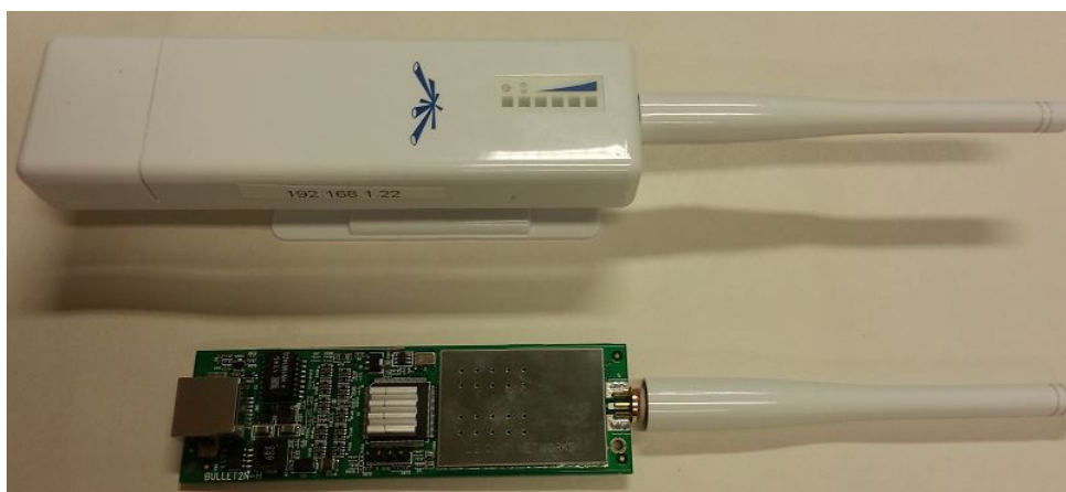
Figure 3.6: The PicoStation M2 HP, with and without its plastic housing.
