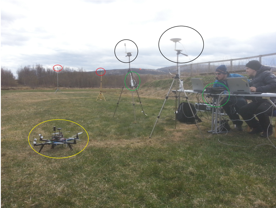
Figure 4.37: Outdoor experiment setup. Red circle shows 2 of 6 Atmel anchors placed around the field. Yellow circle shows one of the hexacopters. Green circle shows the telemetry between the ground control station and the testbed. Also the hexacopter has the same telemetry link. Black circle shows the PiXi base station and the Testbed PiXi antenna. The hexacopter has also the PiXi antenna.
