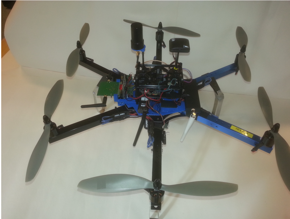
Figure 4.8: The multirotor system. Note that the Atmel reflector (green) and PicoStation (white) are relatively close.
