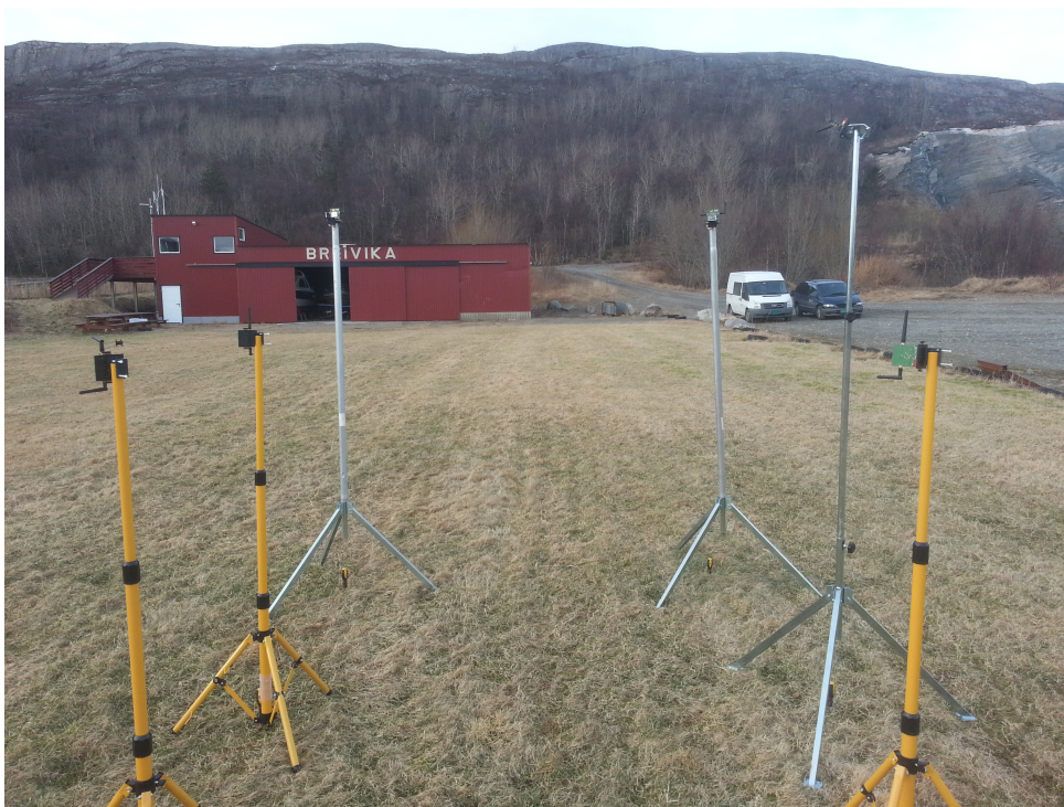
Figure 4.38: Atmel anchors attached to masts during outdoor experiments. Picture is from Agdenes airfield.
