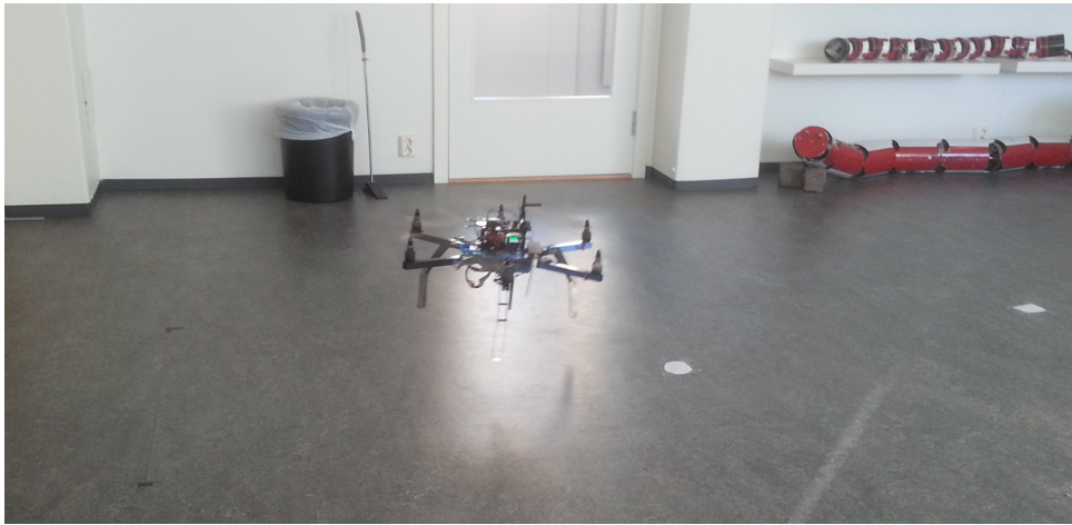
Figure 4.32: Indoor flight with the hexacopter in Robotlab. 6 anchors are used to track the position with the developed EKF while 16 OptiTrack cameras track the system.
