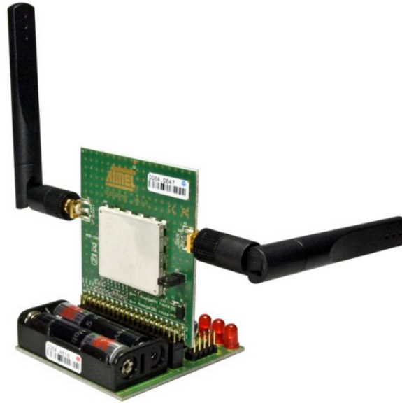
Figure A.1: The REB233SMAD based hardware platform. Image by courtesy of atmel.com
