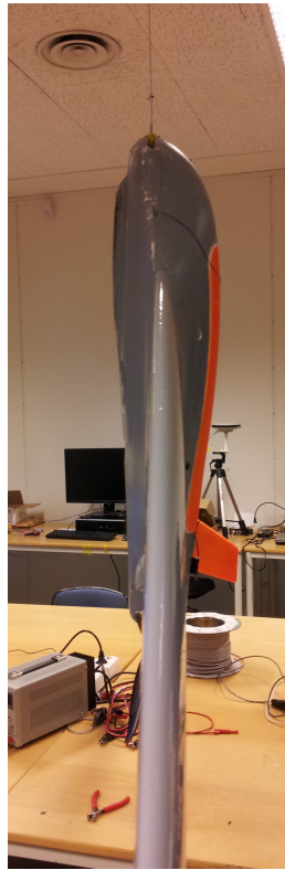
Figure F.4: The setup for the pendulum test for finding I_{zz}
