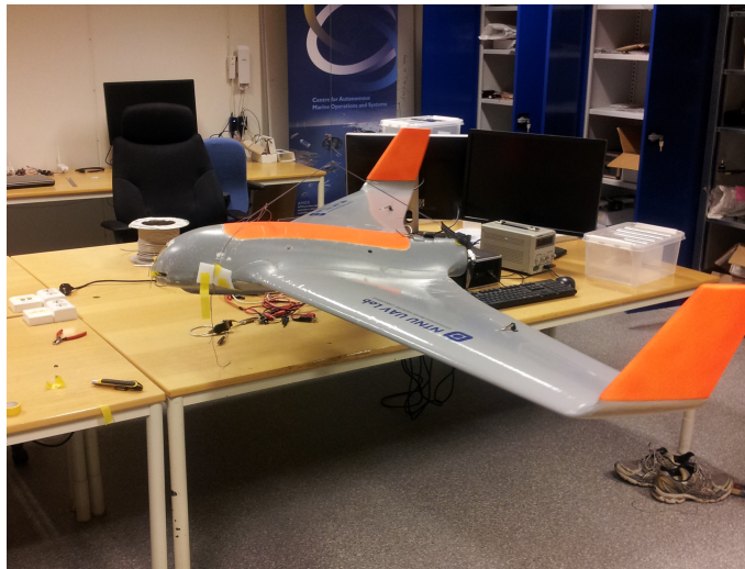
Figure F.3: The setup for the pendulum test for finding I_{xx} and I_{yy}
