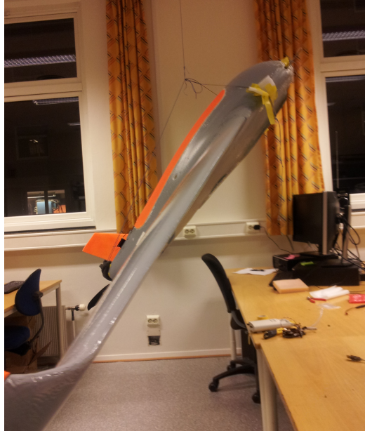
Figure F.2: Setup for performing the pendulum test for finding I_{xz}
