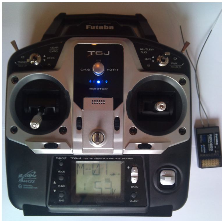
Figure 8.9: Futaba transmitter and receiver - The T6J transmitter and R2006GS receiver
