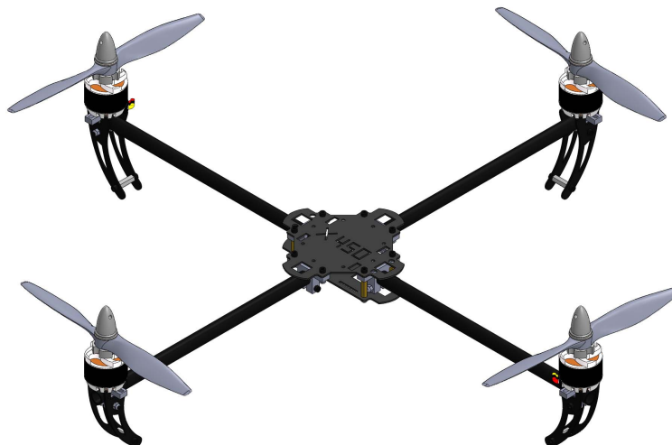
Figure 1.1: Quadcopter - The quadcopter has four propellers with fixed pitch.
