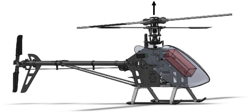
Figure 1.3: Helicopter - Collective pitch - The collective pitch controls the helicopter in the vertical direction. Both blades have equal pitch angle throughout the 360 degree cycle.
