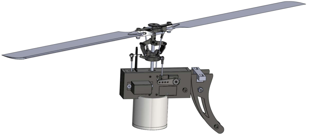
Figure 5.6: Rotor system 1 (250-size) - 3d drawing - Picture of the first designs 3d drawing.
