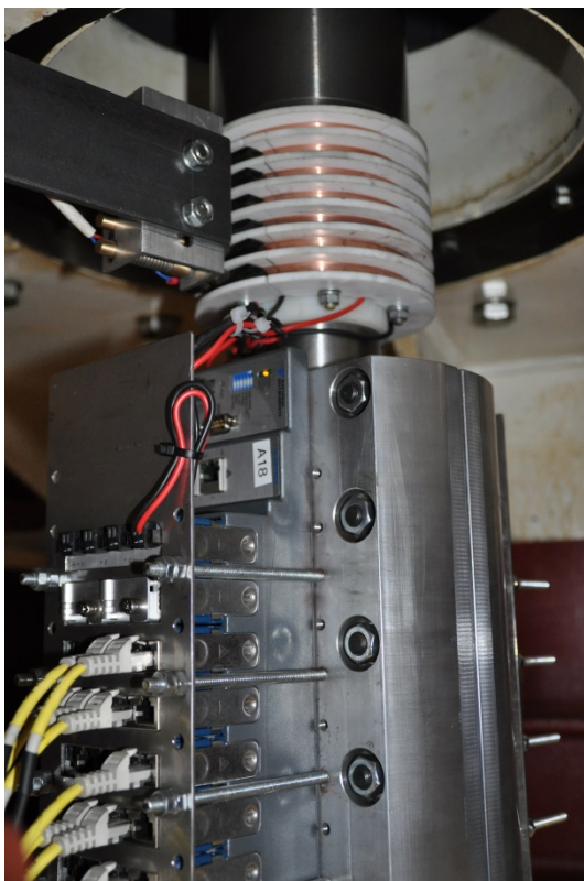
Figure 3.4: cRIO and slip rings mounted on shaft
