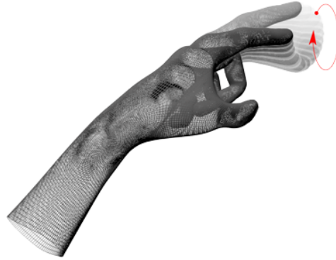
Figure 4.17: How a circular gesture is made according to the Leap Motion’s API. A circle movement is recognized when the tip of a finger draws a circle within the Leap Motion Controller field of view.
