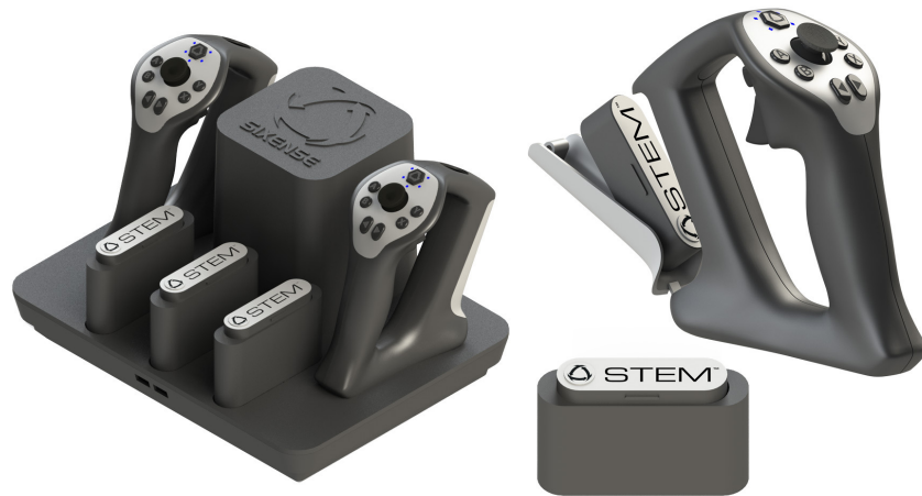
Figure 3.26: The STEM System consists of two motion controllers, wireless motion trackers (STEMs), and a stationary reference for each STEM.
