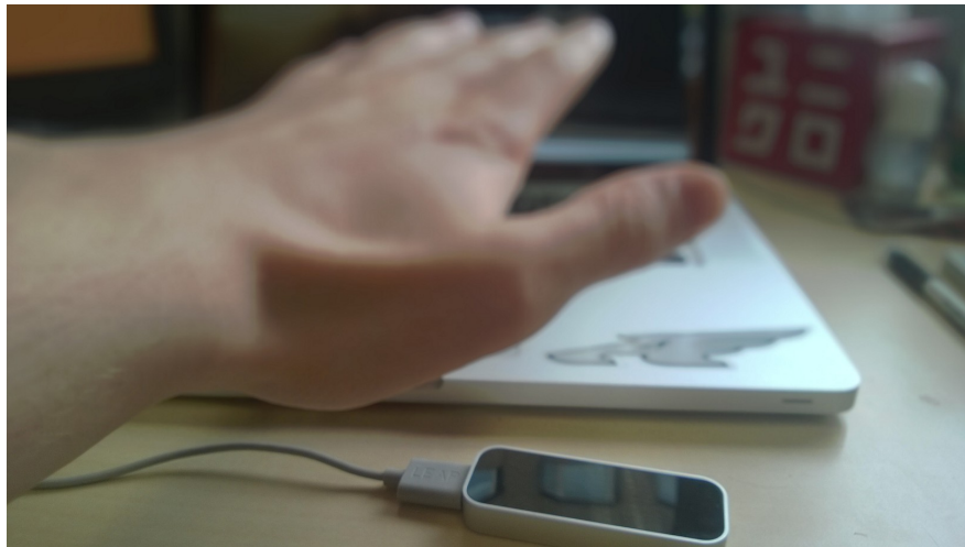
Figure 1.1: Leap Motion is an optic hand tracking device. The device is able to track both hands and all 10 fingers
