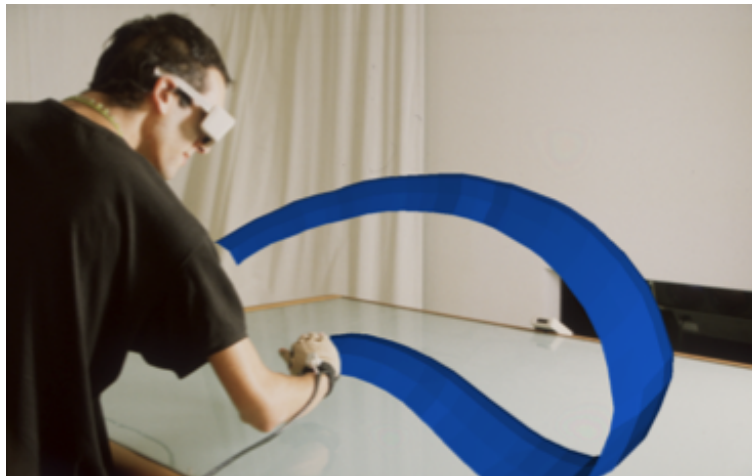
Figure 3.5: Hand motions create shapes which float above the Responsive Workbench. The picture is taken from (Steven Schkolne, 2001)
