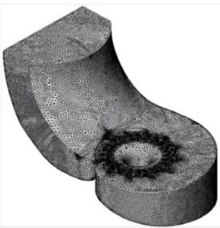
Figure 3.2.1 [8]: Full overview of a simulated mesh, with a 90 degree bend located in close vicinity of the cake-shaped spiral casing
