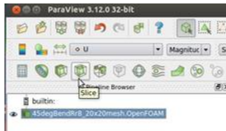
Figure 4.3.1: There is also a Slice button available in one of the upper toolbars.
