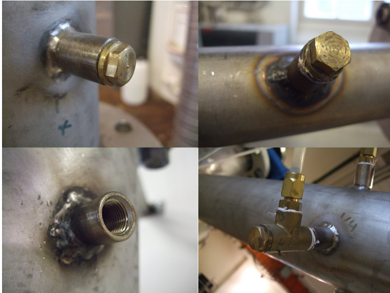
Figure 3.7: Pressure outlets on the rig
