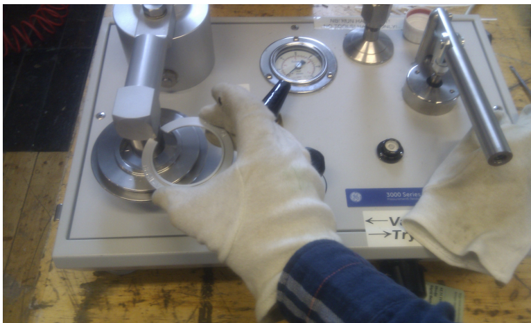
Figure 3.8: Dead weight calibrator
