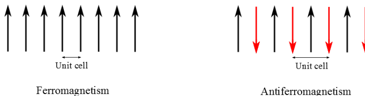
Figure 2.2: Ferromagnetic and antiferromagnetic ordering in one-dimensional magnetic crystals. The magnetic unitcells are indicated with horizontal arrows.
