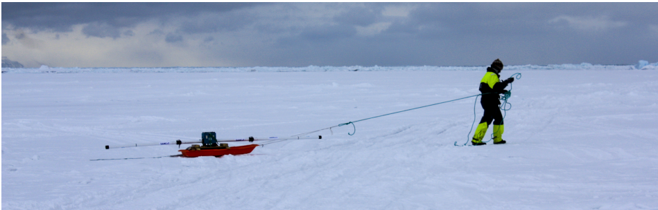
Figure 3.7: Student dragging the EM31 around the ice floe during the stay in Storfjorden
