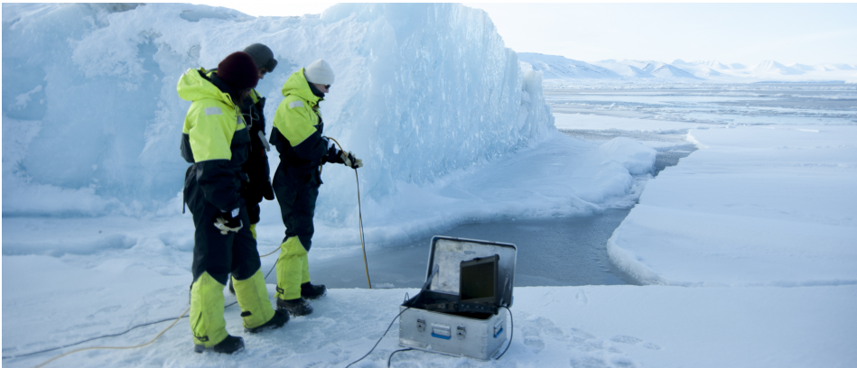
Figure A.1: Use of the EK15 and SBE49 at the iceberg in Storfjorden. The instruments is lowered into the hole. The box contains the power supply and the computer logging the measurements.
