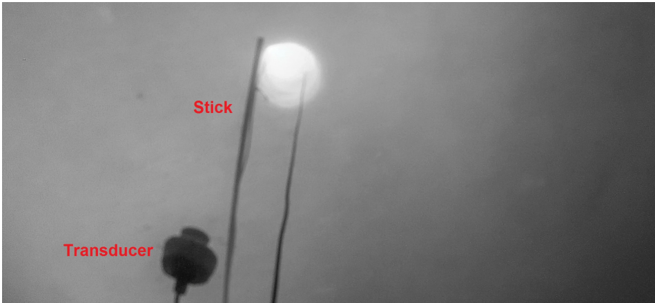
Figure A.2: Picture from the video captured by the underwater camera during operation of the EK15. The picture shows the transducer angled by the current, and the guiding stick being bent.
