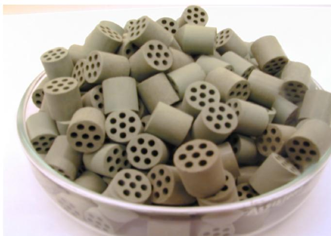
Figure 2.13: Pellets of the catalyst. Image from [2].
