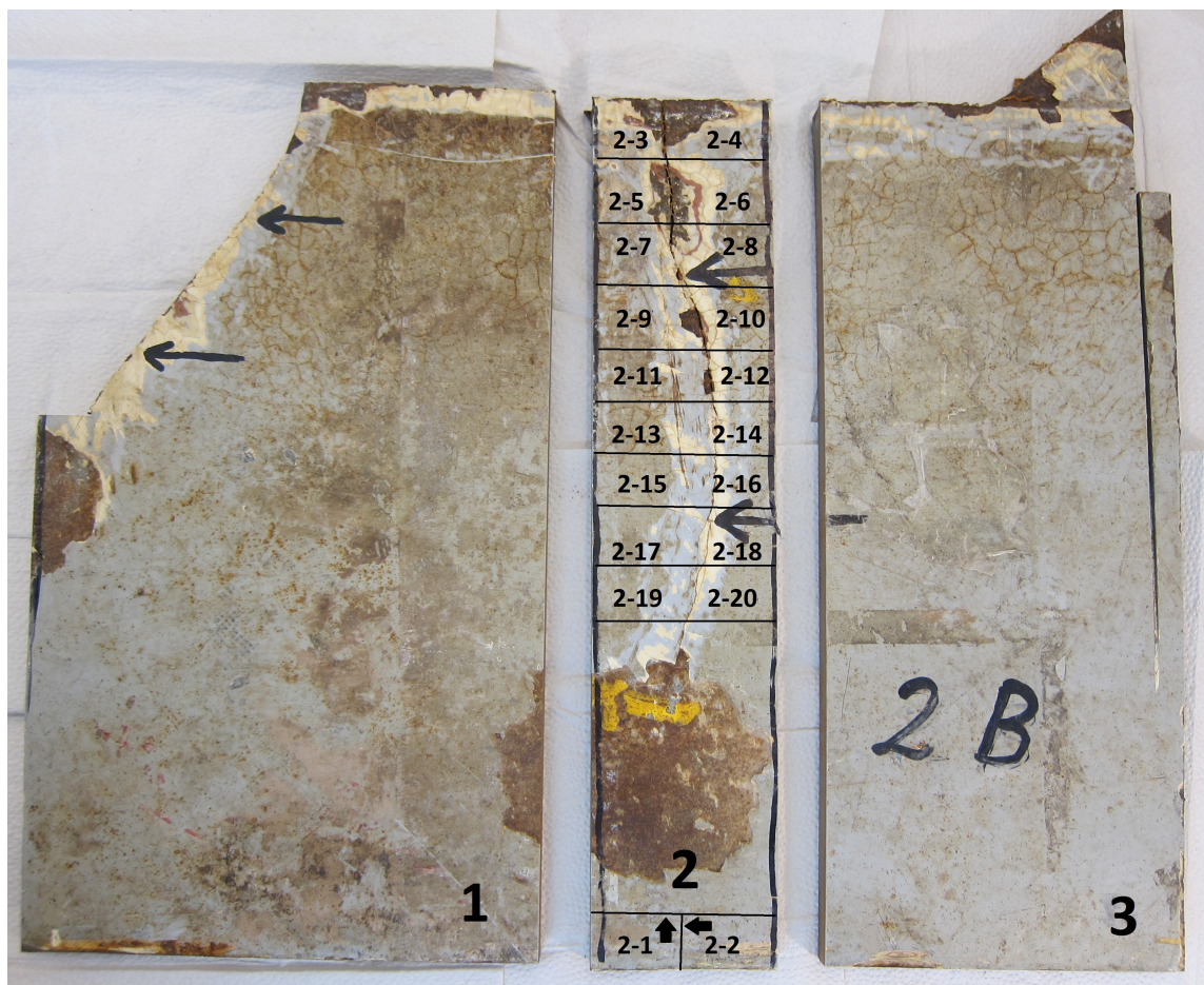
Figure 3.2: The initial sectioning of the material into sections 1, 2 and 3, including the position and numbering of the specimens taken from section 2
