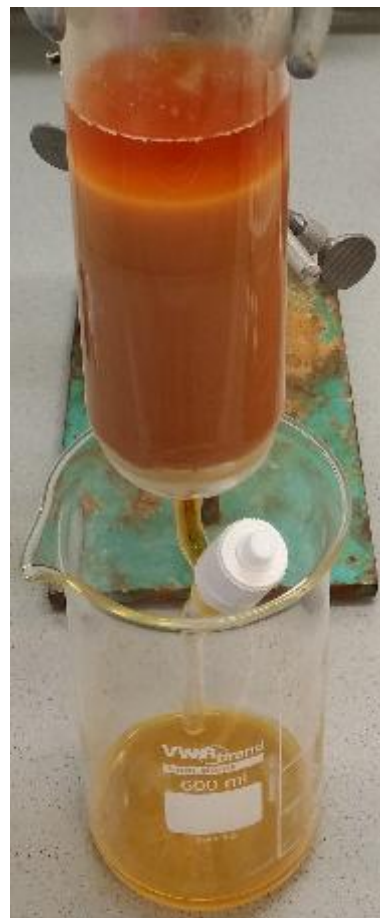
Figure 31: Column with the suspended yeast settling out and plugging the celite disk.
