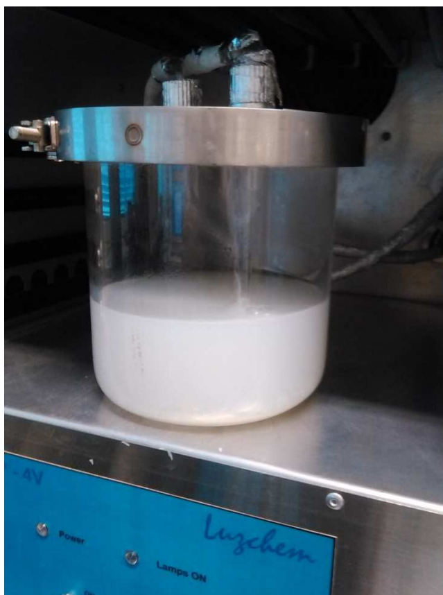
Reactor container during the Argon flow ventilation.
