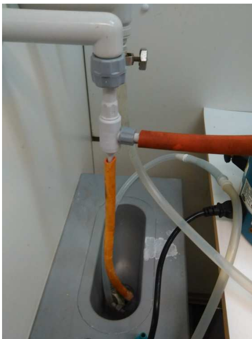
Detail of the Venturi effect vacuum device.
