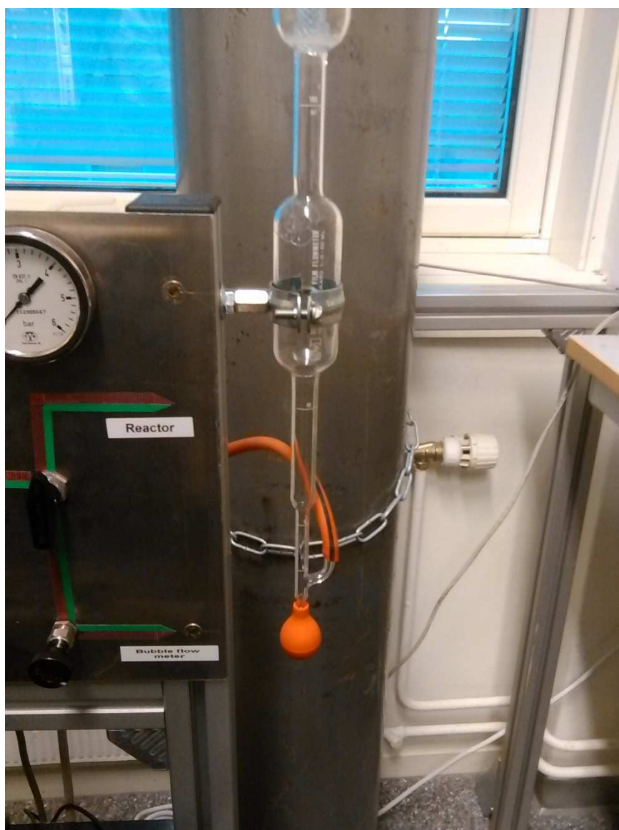
Bubble Flowmeter used for the calibration of the valve
