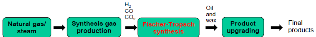
Figure 1.3.1 Main steps in GTL process
