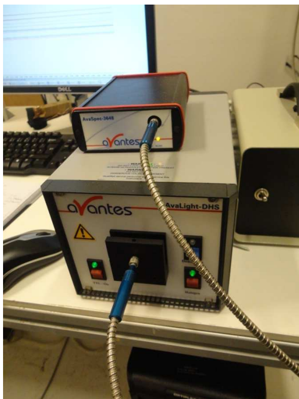
Figure 2.1 Ultraviolet-visible spectrophotometer device used in the experiments.
