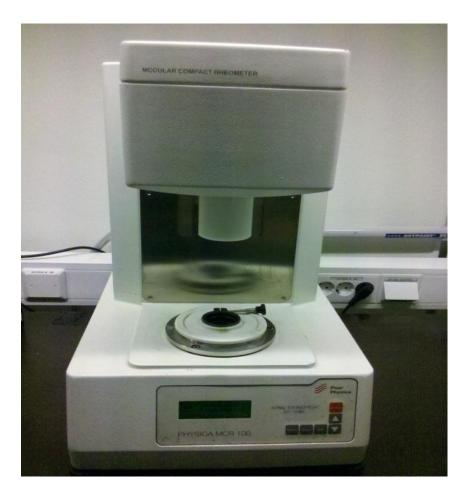
Figure 3.3Pysica MCR 100 rheometer setup for viscosity measurements
