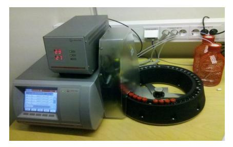
Figure 3.2 Density meter (Anton Paar DMA 4500M)
