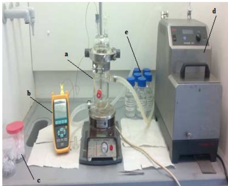
Figure 3.1: Double Walled Glass Vessel attached with Heating/cooling Pump and Digital Thermometer. a: Double Walled Glass Vessel, b: Digital Thermometer, c: Filters, d: Heating/cooling pump, e: Inhibited wax oil solutions
