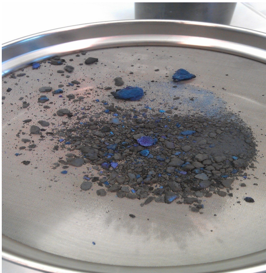
Figure 18: Sample 12.110-a after three hours at 110 °C in the Parr-reactor
