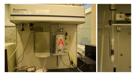
Figure 2.6: Left: Micromeritics ASAP 2020. A: Furnace covering the reactor. Right: Reactor with sample.
