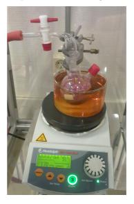
Figure 2.2: Set up for drying of catalysts under vacuum.
