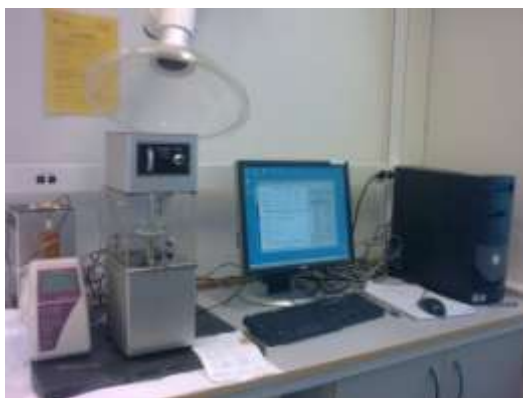
FIGURE 5.12 SIGMA 70 TENSIO METER FOR CALCULATION OF SURFACE TENSION
