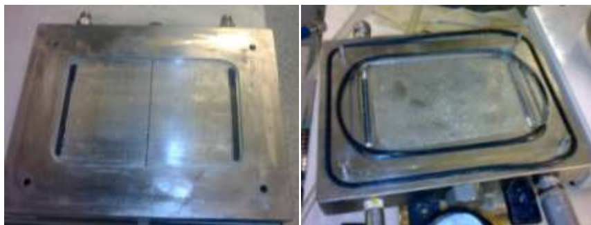
FIGURE 5.6 LIQUID AND GAS CHAMBERS OF MEMBRANE CELL
