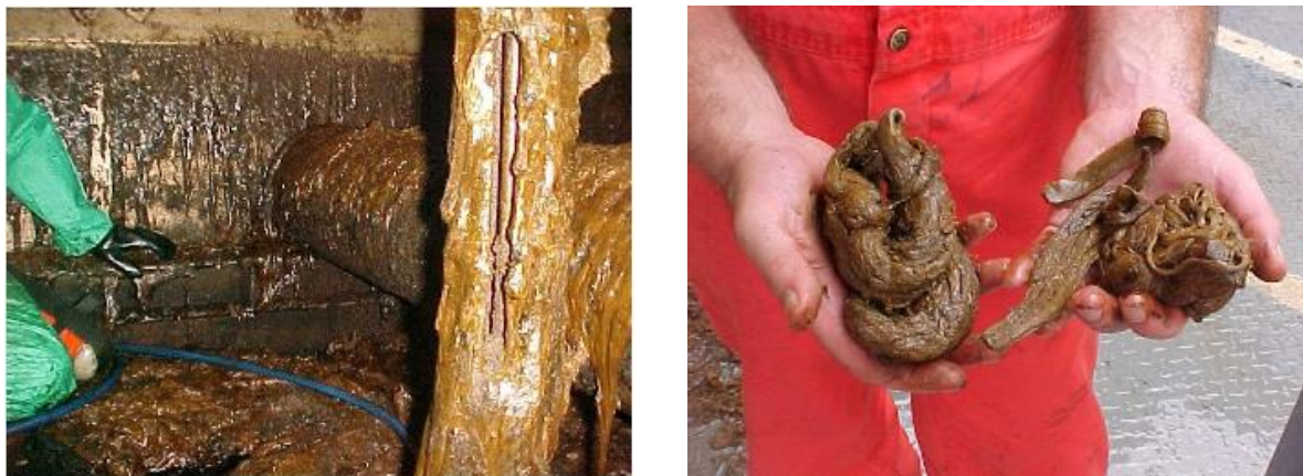
Figure 2 Calcium naphthenate deposits[1]
